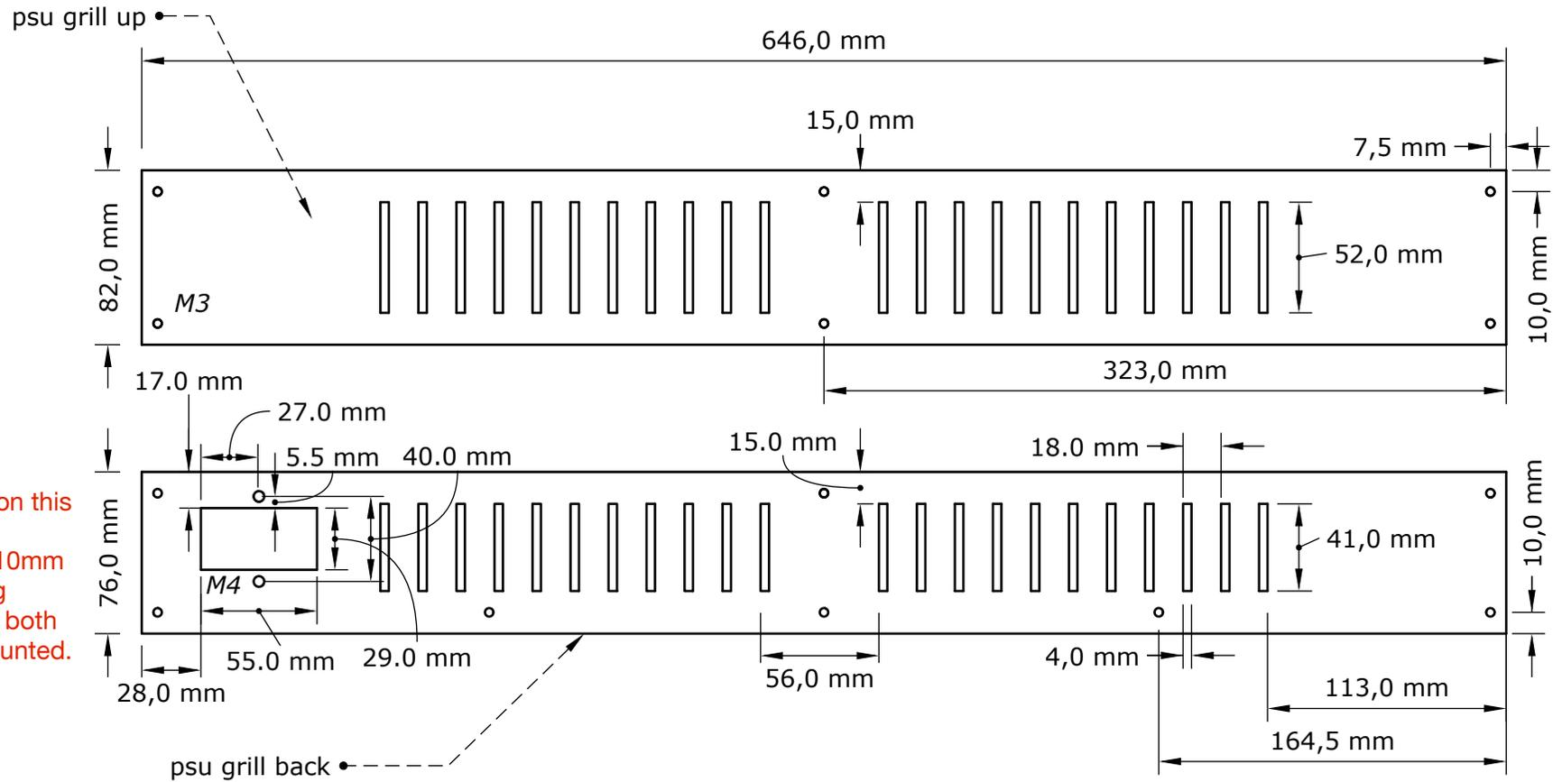
FIXME: The top mounting holes on this panel should be moved down 5-10mm to avoid colliding screws between both panels when mounted.
